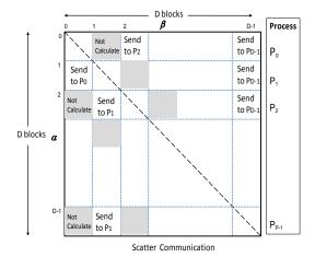
Figure 11. Block Scattered MPI Algorithm: Decomposition (Left) and Scattered Communication (Right) to construct full matrix.
