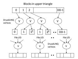
Each D consecutive blocks are merged to form a set of row blocks each with NxD elementsprocess has workload of NxD elements
